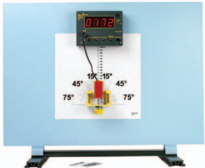
Experiment: Measuring coating thickness, "inno" system
