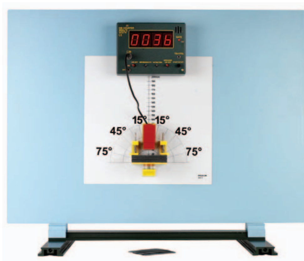
Experiment: Absorption curve of gamma radiation, "inno" system
