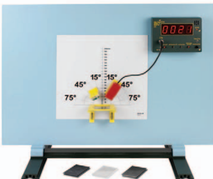
Experiment: Beta backscatter, "inno" system
