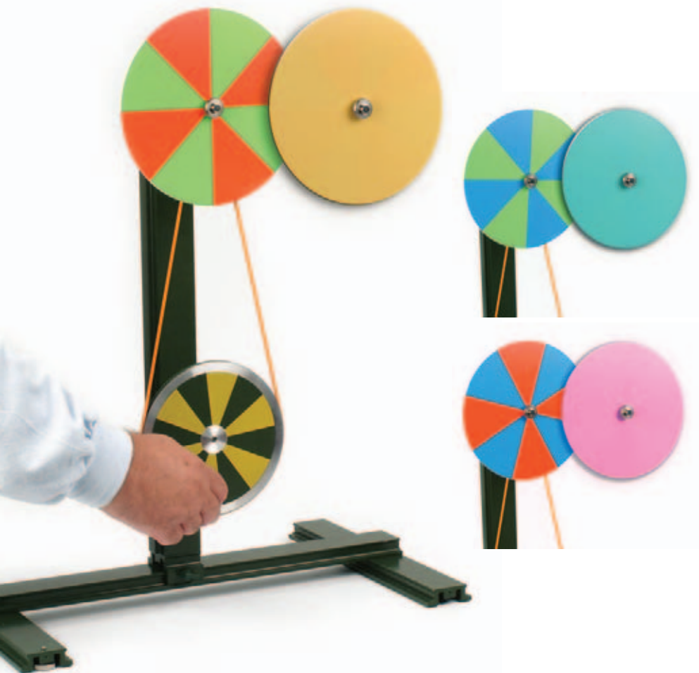
Series of experiments: Mixture of two additive primary colours by rotation, and the results in each case
