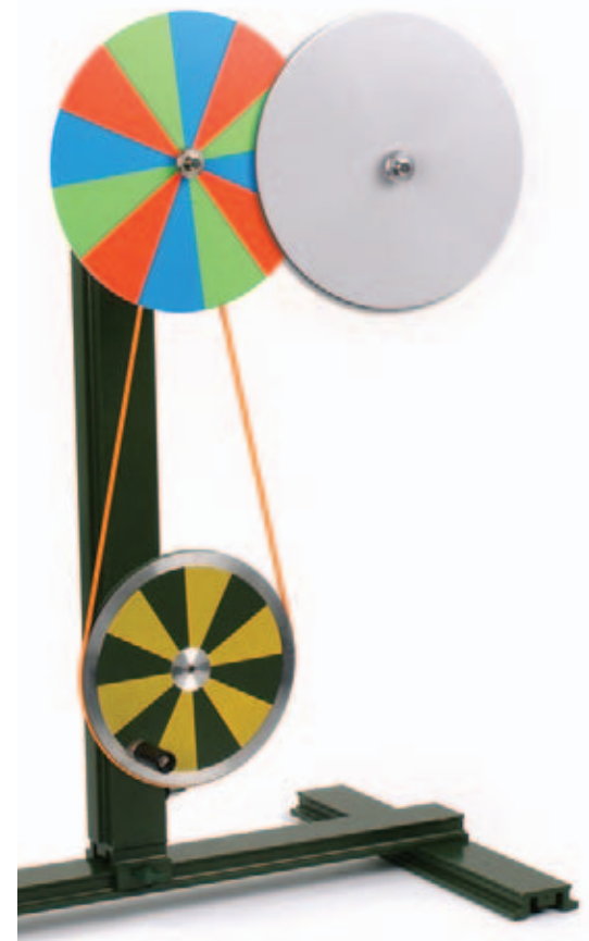
Experiment: Using the red-green-blue colour disk to mix colours, and the result
