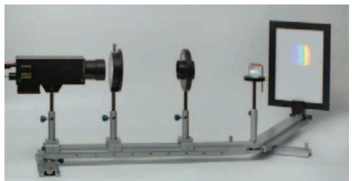
Experiment: Dispersion of white light into spectral colours
