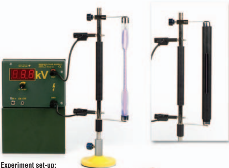
Experiment set-up: Observing the sodium spectrum
