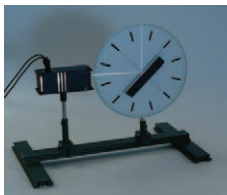
Stand assembly: Optical disc - law of reflection
