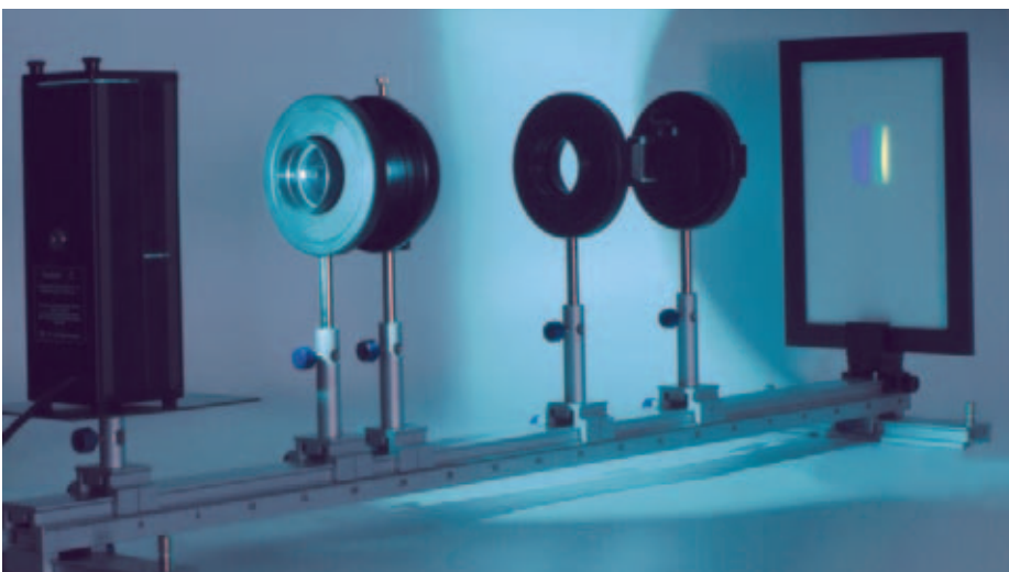
Experiment: Line spectrum of a mercury vapour lamp
