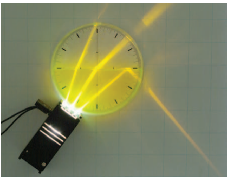
Experiment: Light ray refraction phenomena when passing from water to air at various angles
