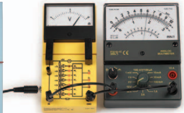
Experiment: Parallel ADC- on a magnetic panel as a demo experiment or horizontally as a student experiment
