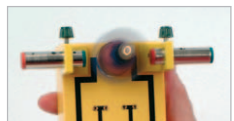
Experiment 090: simple electromotor with two-pole rotor Electromotor module used as a “passive rotating bearing” for a two-pole rotor
