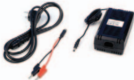
P3130-2P Fixed voltage transformer 12V DC/5.8A Especially suited for supplying power to the AC/DC regulator P3125-2W (P3126-2W) Output voltage: 12 V DC, max. 5.8 A Voltage source: 100 ... 240 V AC/50...60Hz
