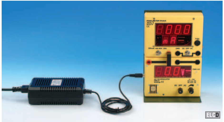
Example for use: AC/DC regulator connected to a fixed-voltage transformer as a power supply and a panelmeter set as an ammeter.
