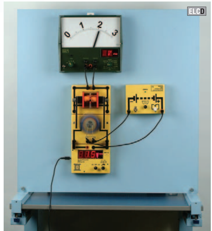
Example for the use of the assembly panel. Demo experiment: ELCD 120 Revolving field generator with electromagnetic rotor
