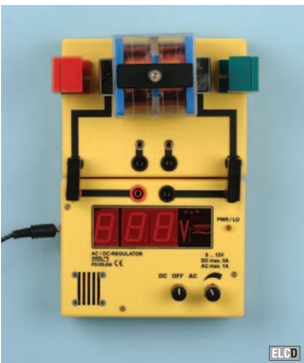
Experiment 117: Simple AC generator - electromotor module used as an “active drive motor” for the rotor coil
