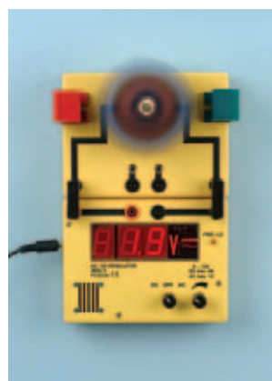
Experiment 117: Simple AC generator - electromotor module used as an “active drive motor” for the rotor coil
