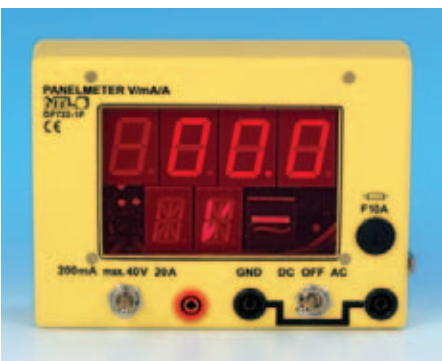
DP722-1P Panelmeter “compact” Demonstration instrument for measuring current and voltage. Display: 3 1/2-digit LED display; digit height 26 mm Measuring ranges: 0 ... 200 mA, 0 ... 20 A, 0 ... 40 V AC/DC See under DE722-1P on page 273 for further technical details.
