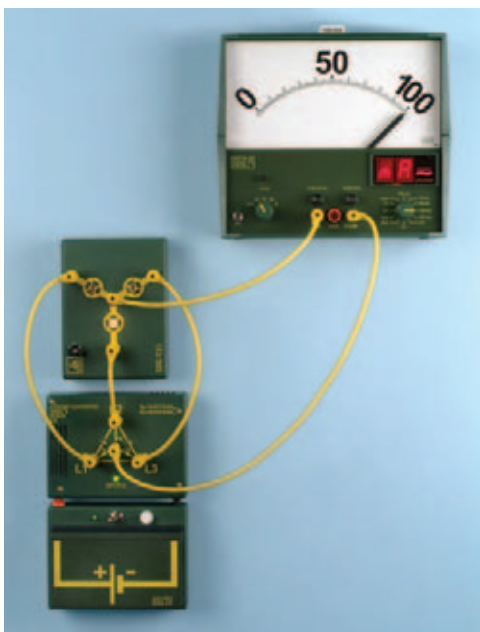
Experiment: Star connection - amperage at the star point (magnetic panel assembly)
