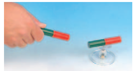
Experiment: Interaction between magnets
