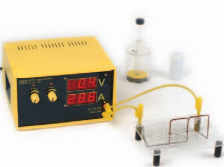
Series of experiments: Field lines produced by various conductor models on an acrylic base
