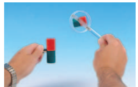
Experiment: Detecting the three-dimensional distribution in space of a bar magnet's field
