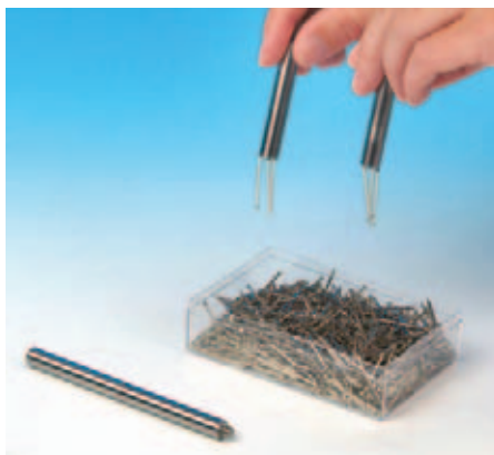
Experiment: Dividing a permanent magnet - identifying the individual magnets
