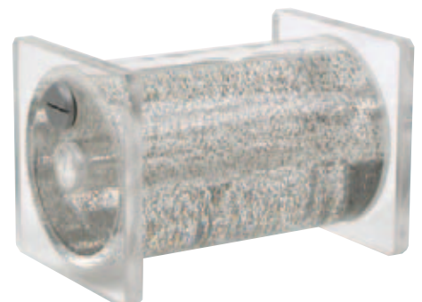
Experiment: Spatially depicting a bar magnet's field
