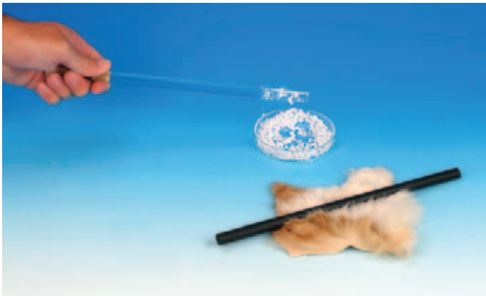
Experiment: Separating electrical charges by means of friction
