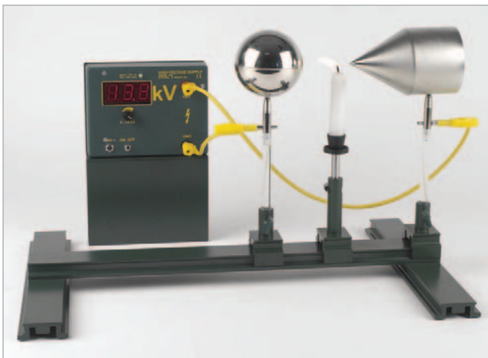
Experiment: "electrostatic wind" - movement of charge to the point
