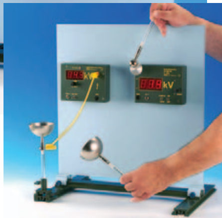
Experiment: Electrical conductors and the distribution of charge - "Cavendish" hemispheres
