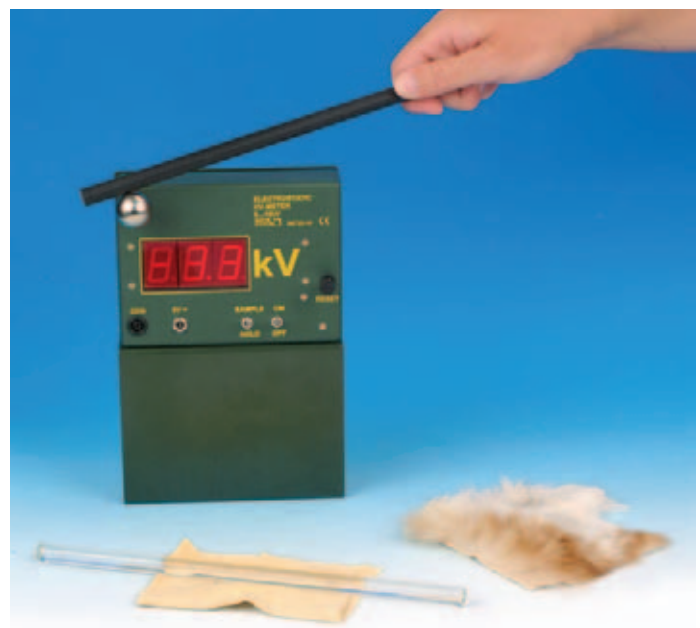
Experiment: Demonstrating voltage using the "inno" static voltmeter
