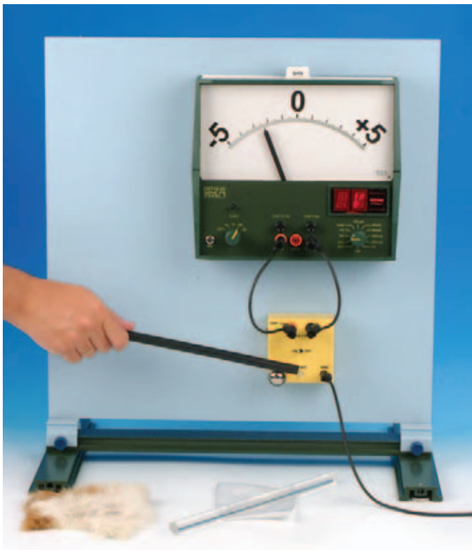
Experiment: The negative charge of the static electricity from hard rubber is displayed - magnetic panel assembly
