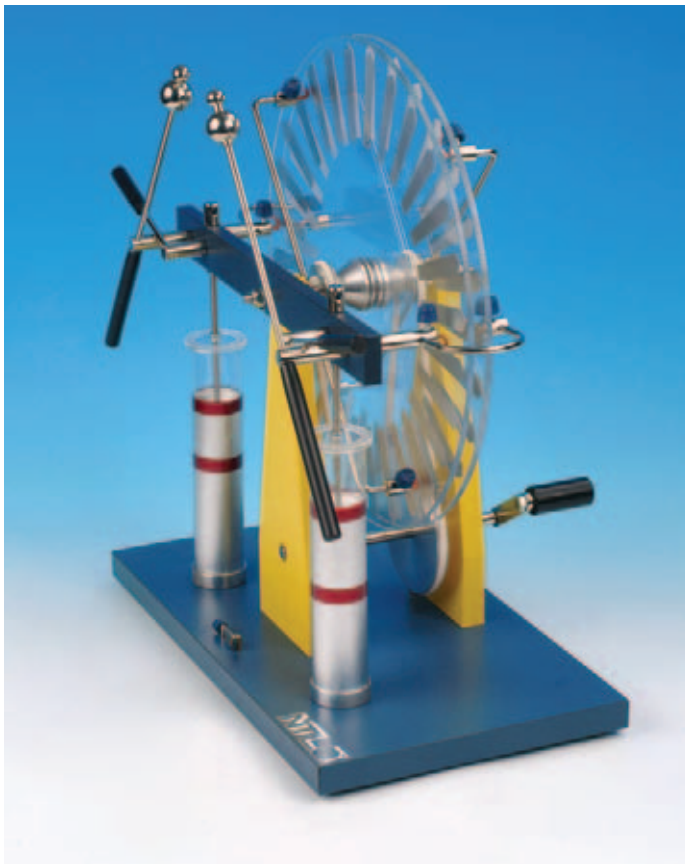
DE523-1A Wimshurst machine Electrical influence machine for generating very high DC voltages Spark length: max. 70 mm Voltage: max. 160 kV Disc diameter: 300 mm Dimensions: 350x200x390 mm
