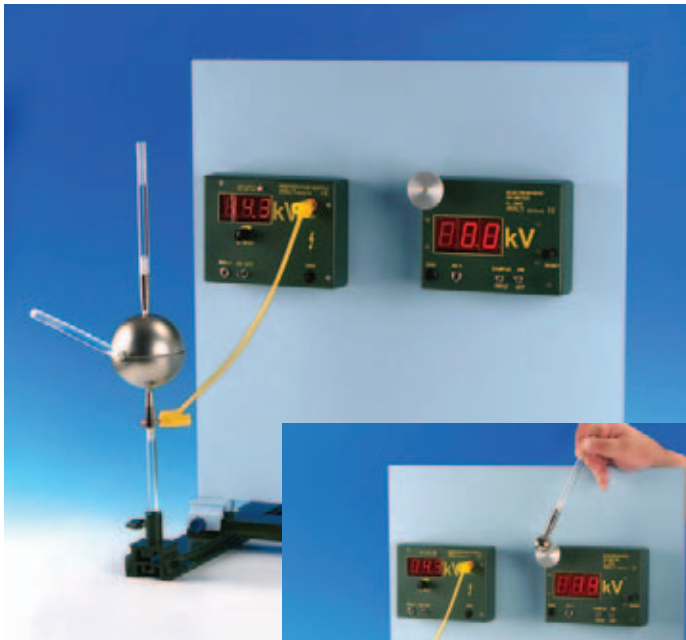
Experiment: Electrical conductors and the distribution of charge - "Cavendish" hemispheres
