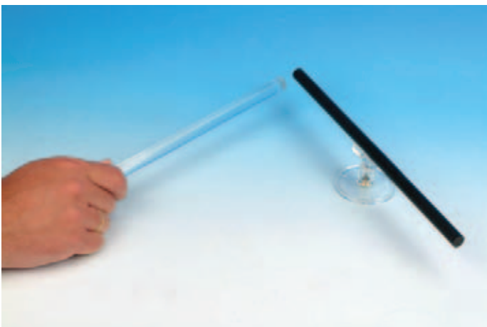
Experiment: Two kinds of electrical charges - hard rubber rod pivoting on needle bearing with base
