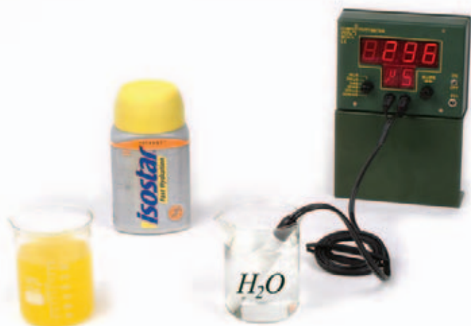
Experiment: Measuring the conductivity of water, with and without table salt, and of an electrolyte beverage
