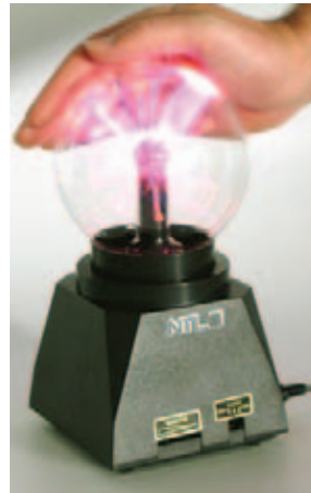
Experiment: Deflecting the flashes resulting from the gas discharge by influencing the external field
