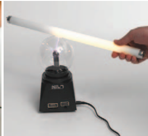
Experiment: Demonstrating the presence of an electrical field using a neon lamp
