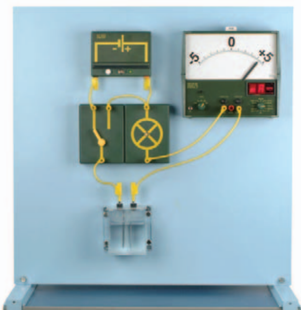
Experiment: Charging and discharging a lead cell ("inno" system) - magnetic panel assembly
