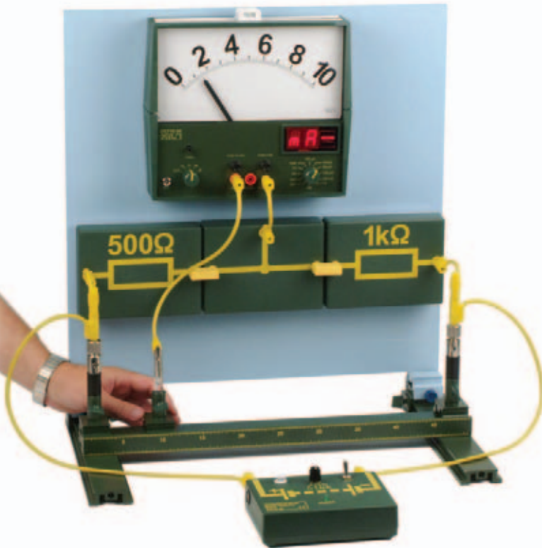
Experiment: Wheatstone bridge circuit ("inno" system) - magnetic panel assembly
