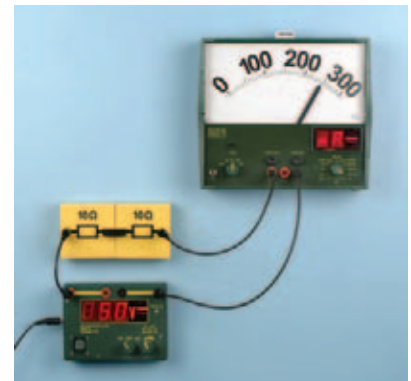
Experiment: Resistors wired in series ("compact" system) - magnetic panel assembly
