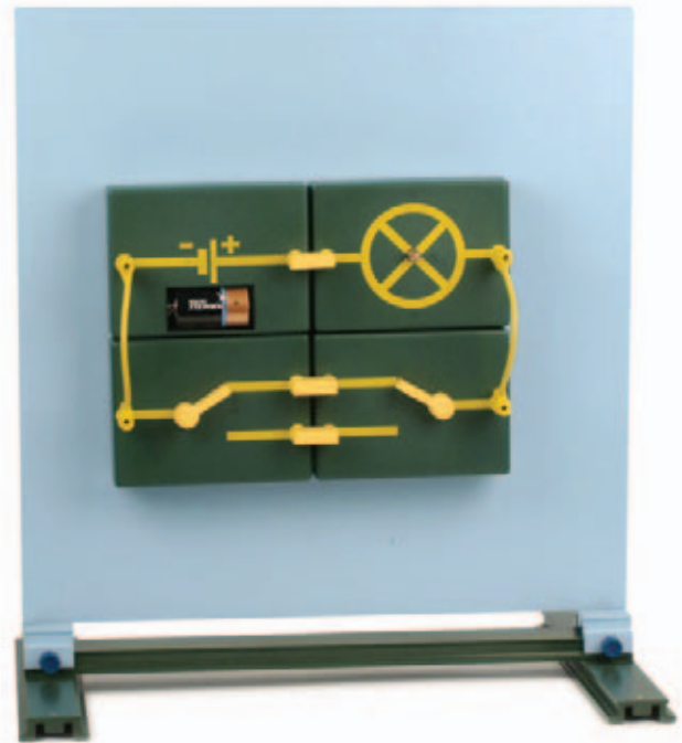
Experiment: Two-way circuit ("inno" system) - magnetic panel assembly
