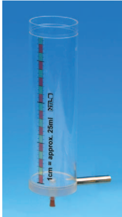
P1412-1A 500 ml drainage beaker on support
