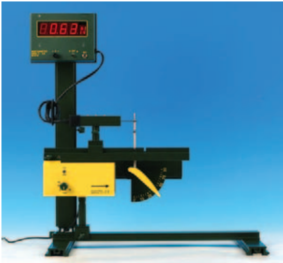
Experiment: Lift under an aerofoil
