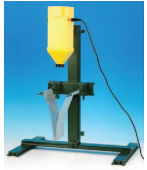
Experiment: Aerodynamic paradox with two curved aluminium sheets
