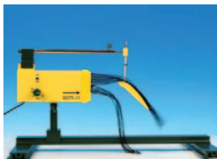
Experiment: Flow patterns at different aerofoil positions
