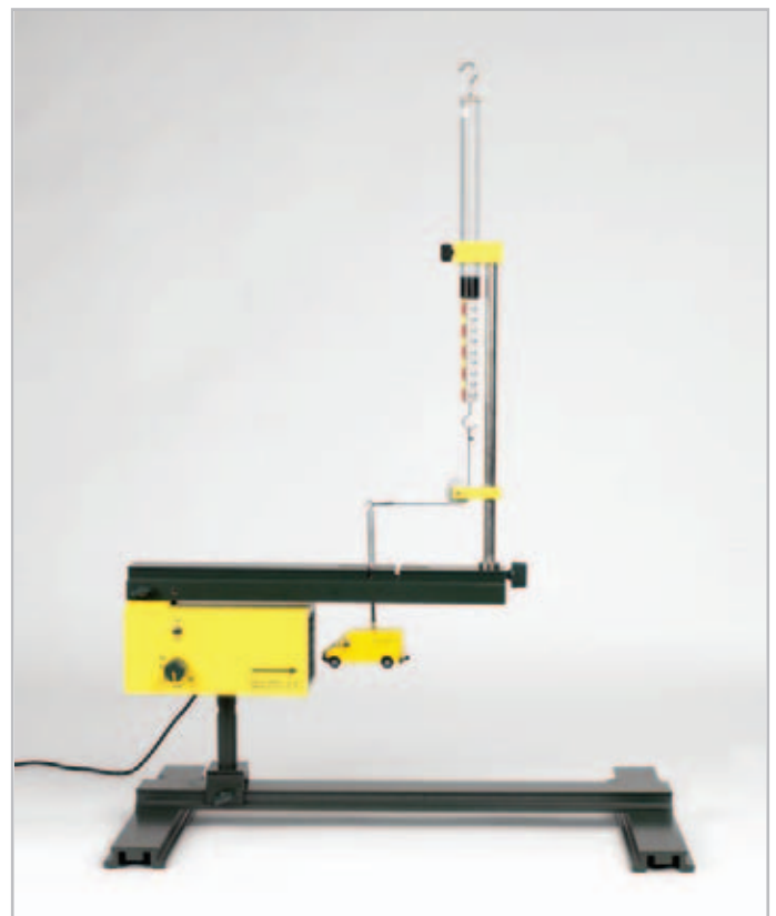
Experiment: Measuring the aerodynamic resistance of the model delivery van
