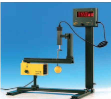
Aerodynamic body; Ball with smooth surface
