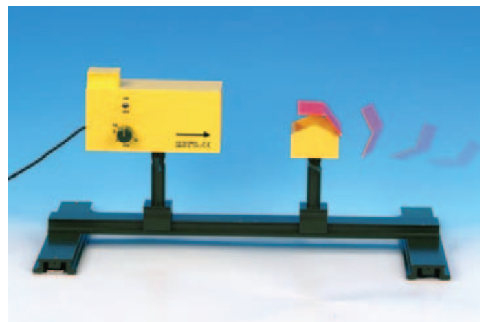
Experiment: Slightly sloped house roof being blown off by a strong airflow (storm)
