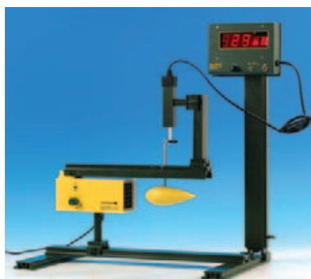
Aerodynamic body; Aerodynamic profile of a smooth surface
