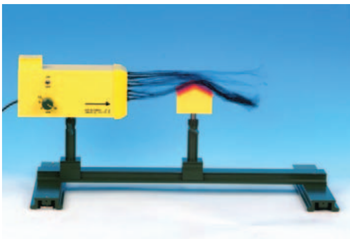
Experiment: Flow pattern over a roof
