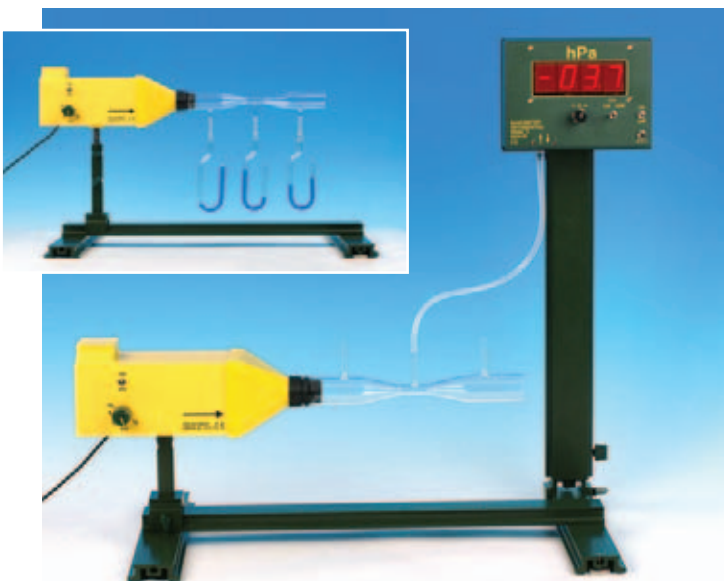
Experiment: Pressure within an air stream - Venturi tube
