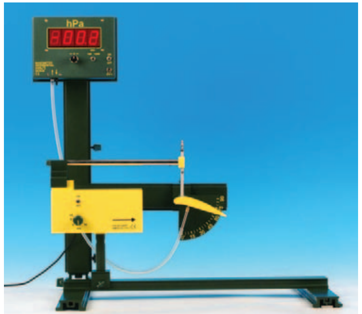
Experiment: Distribution of pressure over an aerofoil
