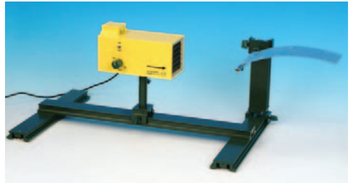
Experiment: Lift in an air stream
