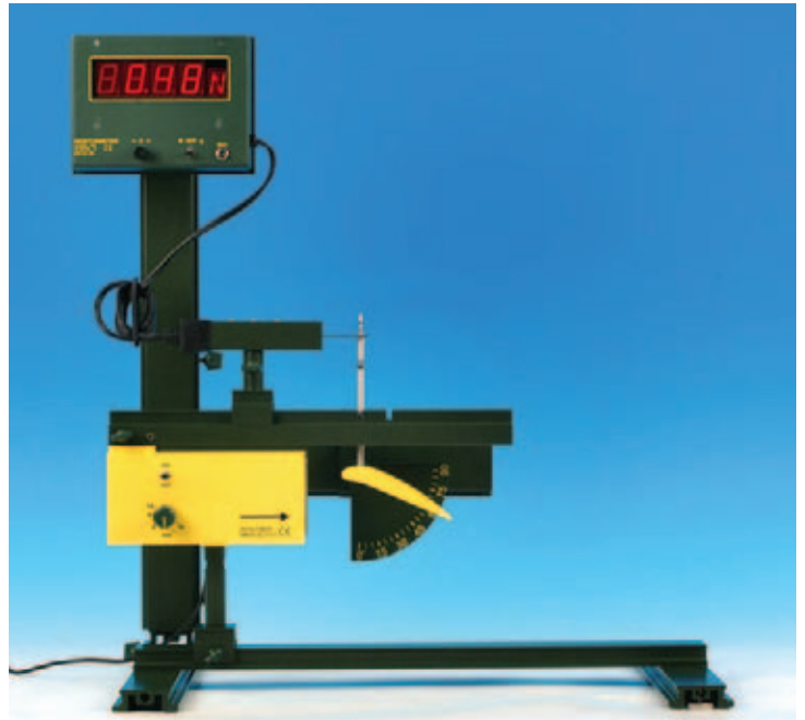
Experiment: Lift under an aerofoil
