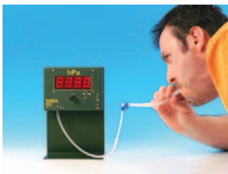
Experiment: Measuring low pressure in an atomizer
