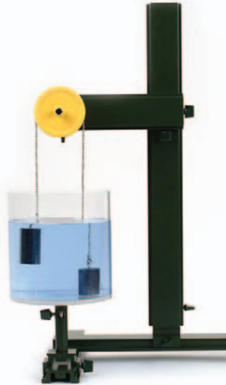
Experiment: Buoyancy of objects with different densities, demonstrated with the bodies of equal mass DM140-2C
