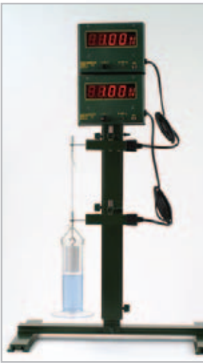
Experiment: Measuring the force of buoyancy - newtonmeter "inno"
