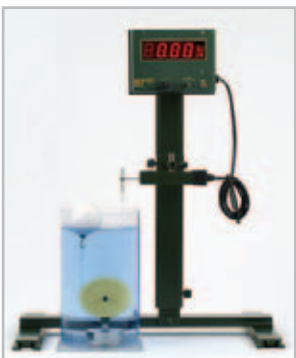
Experiment: Measuring the buoyancy of a Styrofoam ball
