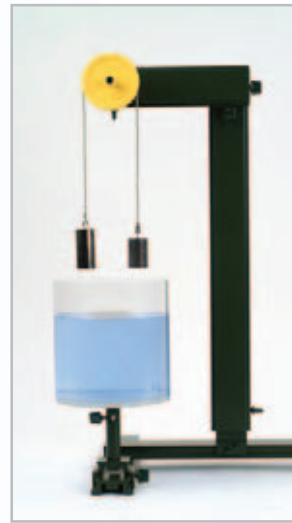
Experiment: Buoyancy of objects with different densities, demonstrated with the bodies of equal mass DM140-2C
