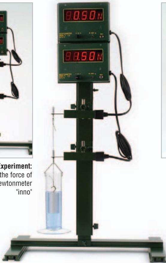
Experiment: Buoyancy of objects with different densities, demonstrated with the bodies of equal mass DM140-2C
