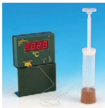
Experiment: Rise in pressure - rise in temperature
