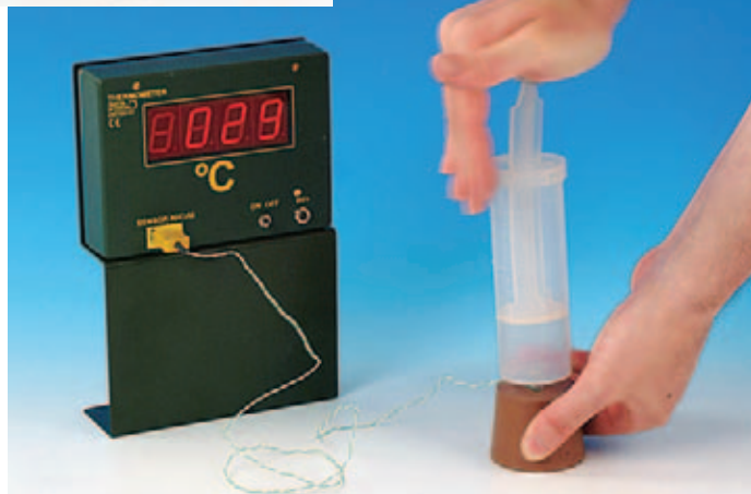
DM113-1H Syringe sampler with plunger 150 ml, plastic With tapped hole for c-hook DS102-3S Dimensions: D=46 mm, L=205 mm C7320-6S Rubber stopper 36/44/40 mm , with hole closed at one end C7416-1B Pinchcock, Mohr, large C7445-7S Hose, silicone, D=7/9 mm, L=100 cm
