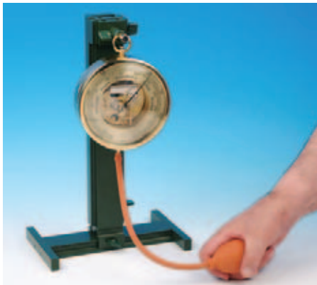
Experiment: Measuring air pressure using a barometer
