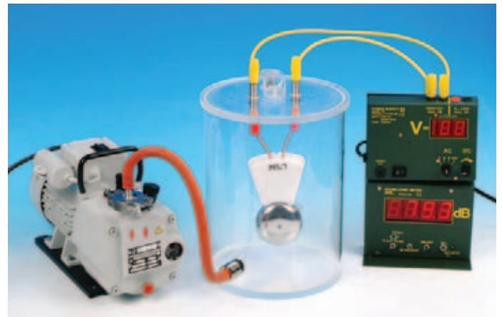
Experiment: Transmission of sound in a vacuum
