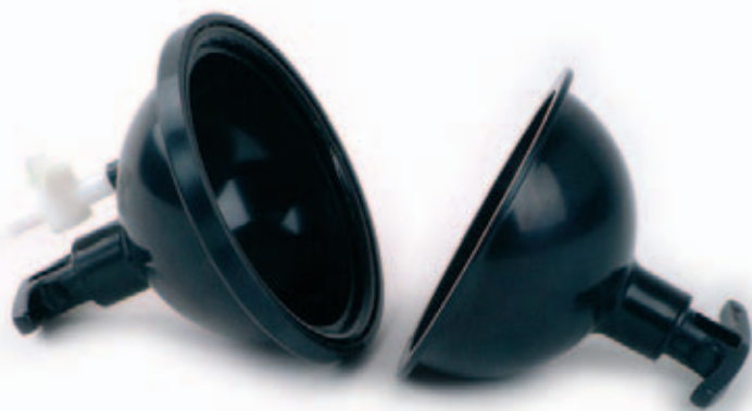
DM550-1M Magdeburg hemispheres, pair For demonstrating the effect of atmospheric pressure (historical experiment by Guericke); 2 plastic half-spheres with handles, fitted with rubber sealing gasket, with stopcock Diameter: 100 mm
