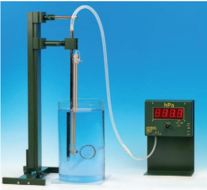
Experiment: Measuring hydrostatic pressure using the Hartl capsule and the "inno" differential manometer
