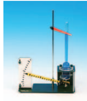
Experiment: Hydrostatic paradox
