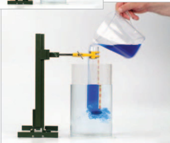
Experiment: Hydrostatic pressure in an upwards direction
