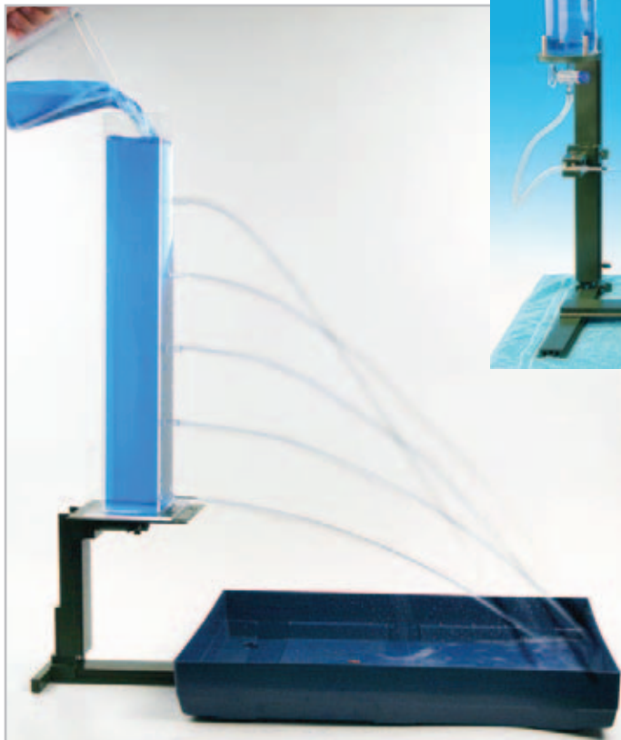
Experiment: Lateral pressure and flow velocity of discharge
