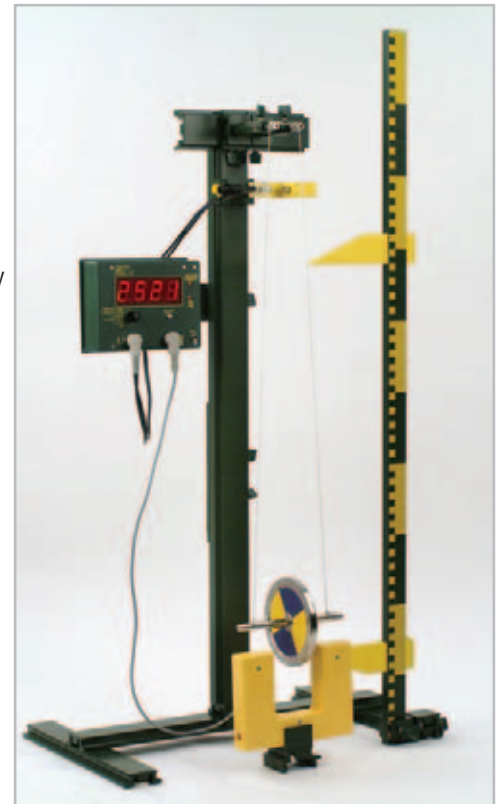
Experiment: Conservation of energy in Maxwell's rod (with time being recorded)
