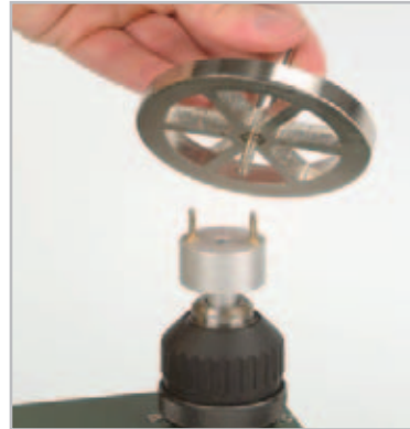
Detail: Gyroscope driven by drive shaft clamped in drive motor DS403-2S
