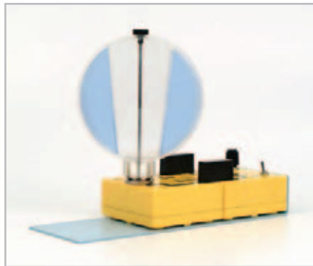
Experiment: High rotational speed causes the water in the cell to "divide"
