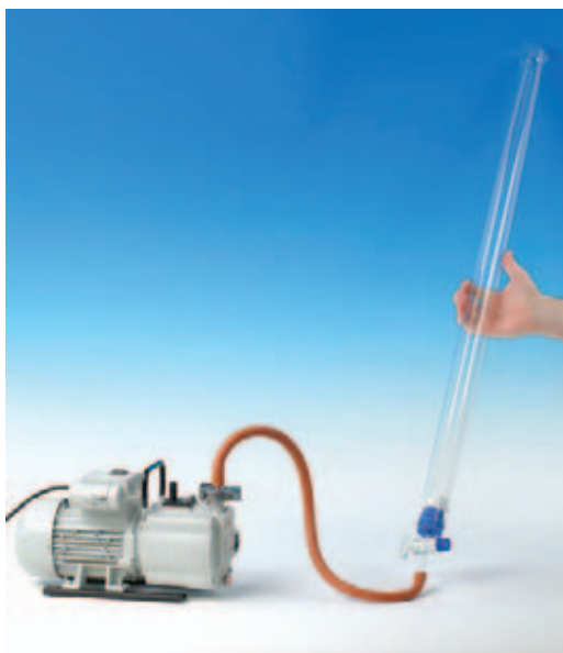
Detail: Free-fall tube with stopcock for evacuating and falling objects
