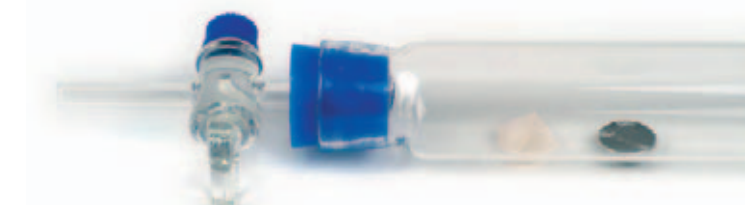
Detail: Free-fall tube with stopcock for evacuating and falling objects
