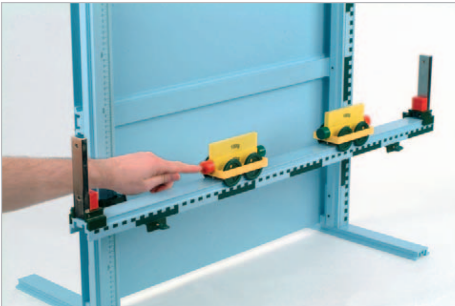
Experiment: Conservation of momentum (on the assembly panel)
