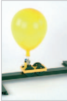
Experiment: Propulsion by airflow (on stand rail)
