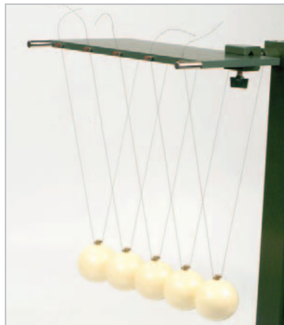
DM750-5K Ball collision assembly, large 5 plastic balls, D=60 mm, bifilar suspension from plate, adjustment screw on one side, suspension plate with 2 support pins, D=10 mm, L=40 mm Pendulum length: 300 mm Dimensions of suspension plate: 300x150 mm
