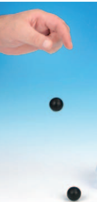
DM810-1H Happy / unhappy balls Two look-alike balls of varying elasticity Diameter: 24 mm each
