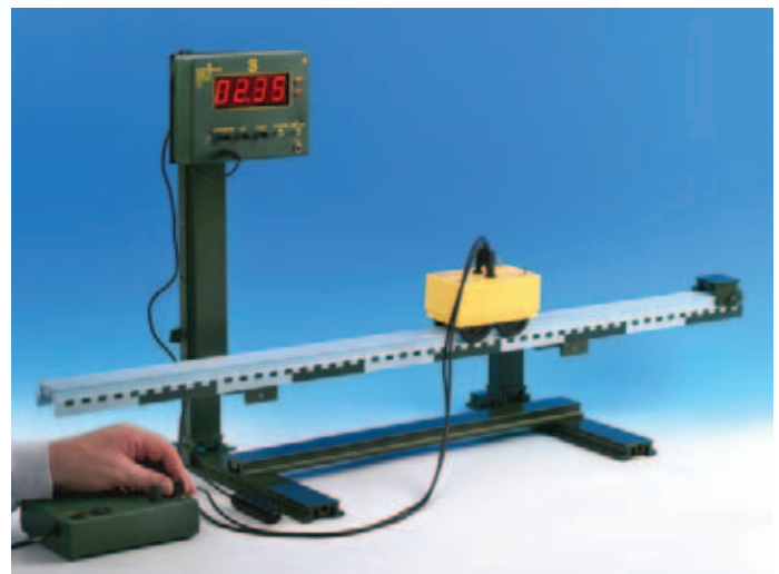
Experiment: Non-uniform linear motion, measurement of average velocity using stopwatch "inno"
