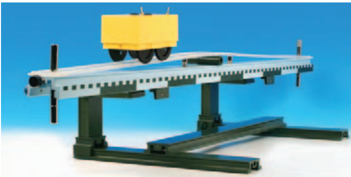
Experiment: Up- and downhill motion (conversion of energy) Universal rail DS101-4B with flexible track DS101-2A, supports DS101-3A and trolley with motor DM300-1A
