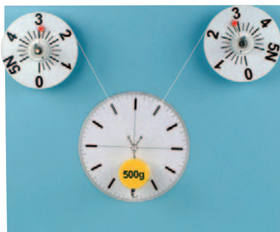
Experiment: Parallelogram of forces, magnetically mounted on assembly panel
