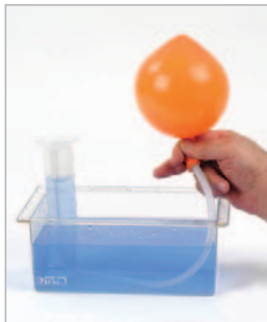
Experiment: Determining the volume of air in a balloon
