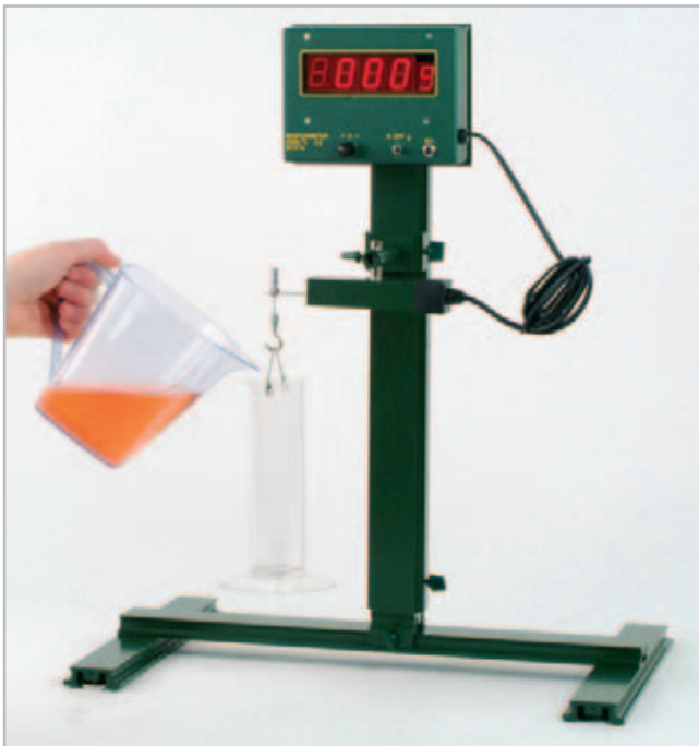
Experiment: Determining the density of a fluid
