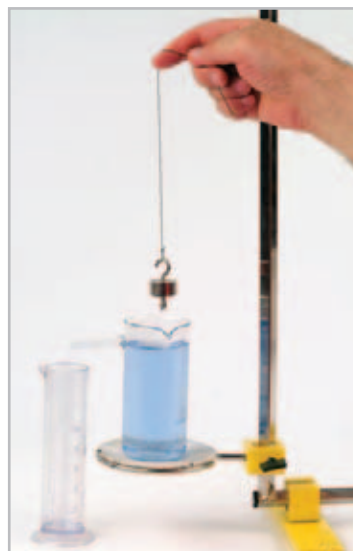
Experiment: Determining the volume of a solid body
