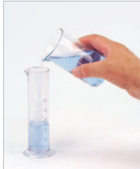
Experiment: Determining the volume of a beaker with a graduated cylinder
