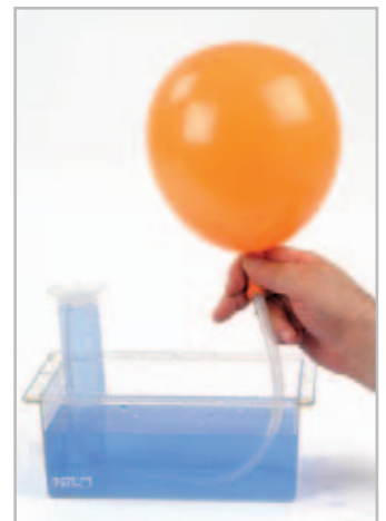
Experiment: Determining the volume of air in a balloon
