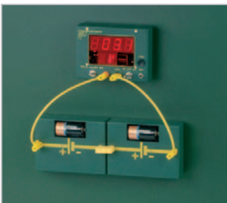
Experiment: Panel, green - sources of voltage connected in series
