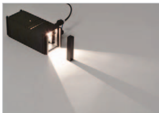
Experiment: Shadows from a halogen lamp
