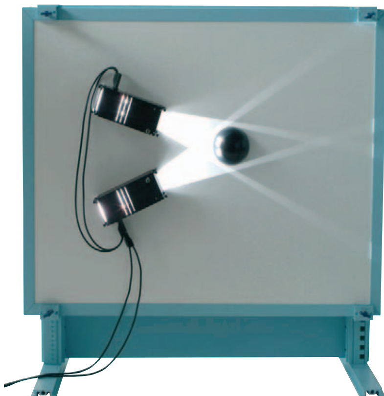
Experiment: Back of demo plug-in panel for electricity DE920-1A as a magnetic optics panel - umbra and penumbra
