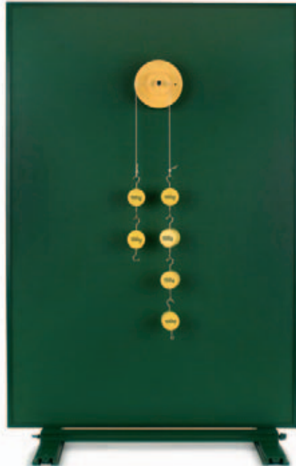
Experiment: panel, green - double wheel and axle
