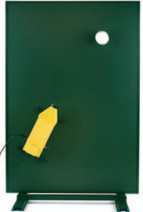
Experiment: Panel, green - dynamic pressure in an air stream
