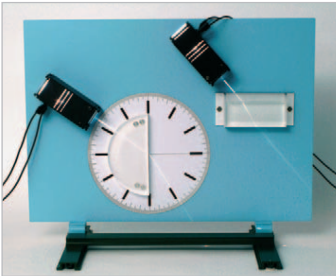
Experiment: Optics - angles of incidence and refraction
