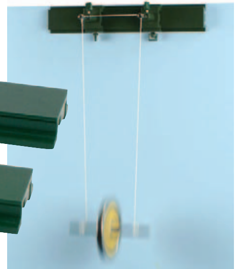
Experiment: Conservation of energy in Maxwell's Wheel
