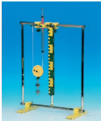
Experiment: Movable pulley
