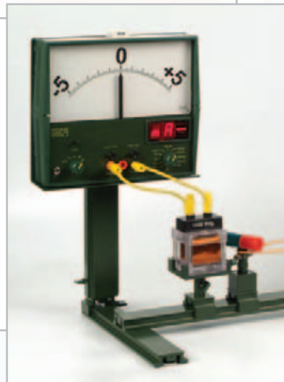
Experiment: Electromagnetic induction - periodic change in the magnetic field
